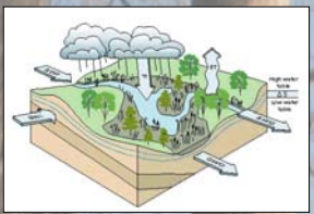
Fig. 1 The inputs and outputs of water in a wetland system: Inputs: groundwater, precipitation, surface flow. Outputs: evaporation, transpiration, groundwater & surface outflow.
