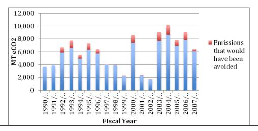
Figure 1.5 Annual Heating Emissions if all Fuel Oil was replaced with Natural Gas.
