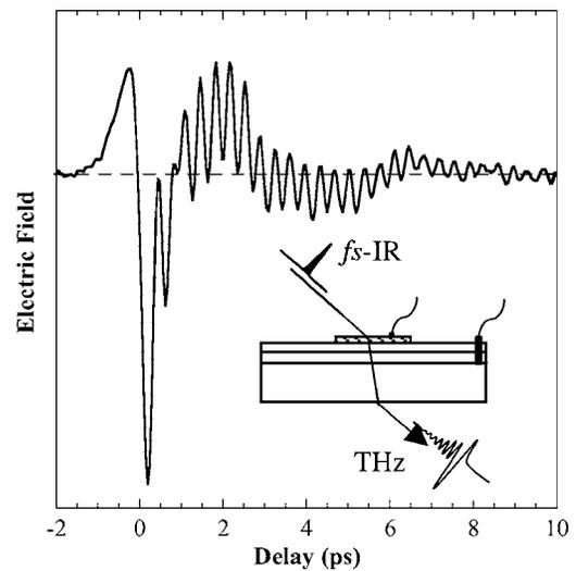
FIG. 1. Terahertz emission from our PQR ( $T = 4.2$  K,  $V_g = -1.0$  V,  $h\nu = 1.55$  eV). Intersubband charge oscillations are observed following impulsive optical excitation at  $t = 0$ . Inset shows experimental geometry.
